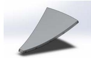
Fig.5 Trapezoidal reflective petal of solar parabolic concentrator
