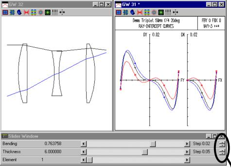
Once again, the up/down arrows on the right hand side of the slider bar window adjusts the precision and range of the sliders themselves. This demo allows the student to virtually bend the lenses of a triplet. By adjusting the sliders, the student can switch which lens is being controlled and attempt to re-balance the system aberrations by observing the ray intercept curves (a.k.a. transverse ray aberration plots).
