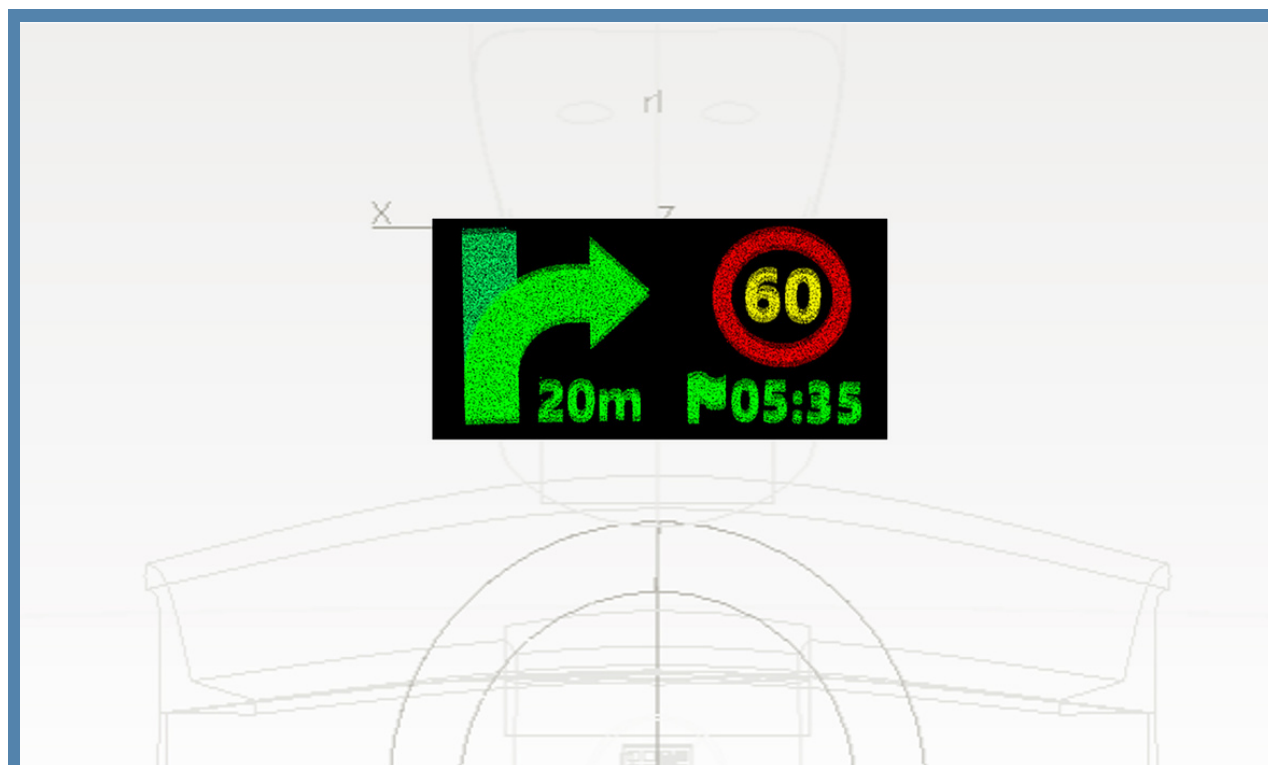
Figure 13: Blurry, double image shown with Photorealistic Rendering
